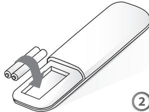
Insert two brand new batteries (7#), and position the batteries to the right electric poles (+ & -).
